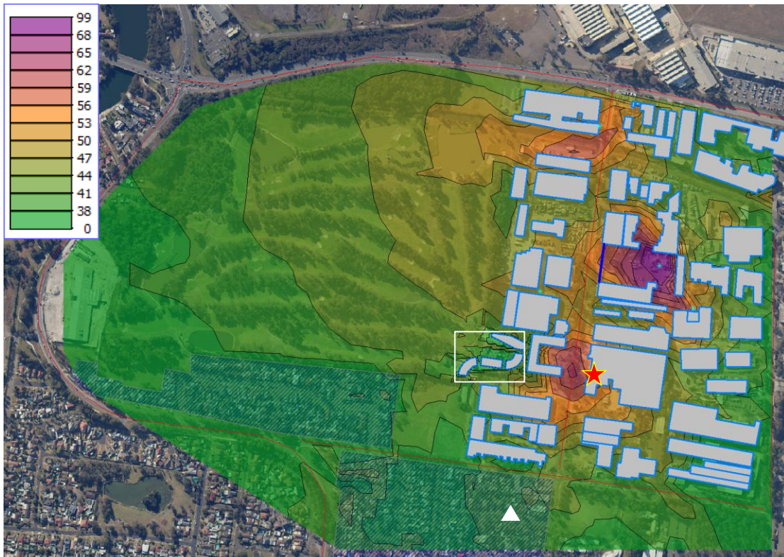
Figure 5. Noise map of L_{Aeq,15min} levels showing daytime cumulative noise levels from existing and future industrial noise sources at receivers at 4 m above ground and on facades of proposed apartments. (Western view in 3D)
